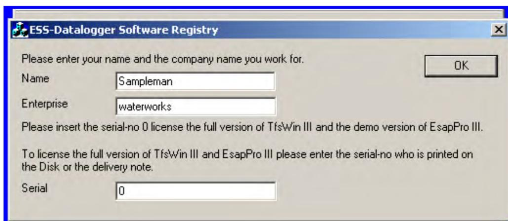
If TfsWin III is used without EsapPro III, the preset „0“ should be confirmed. When EsapPro III was acquired, the serial number, mentioned on the delivery note, must be entered instead of zero. Now EsapPro III is licensed.
