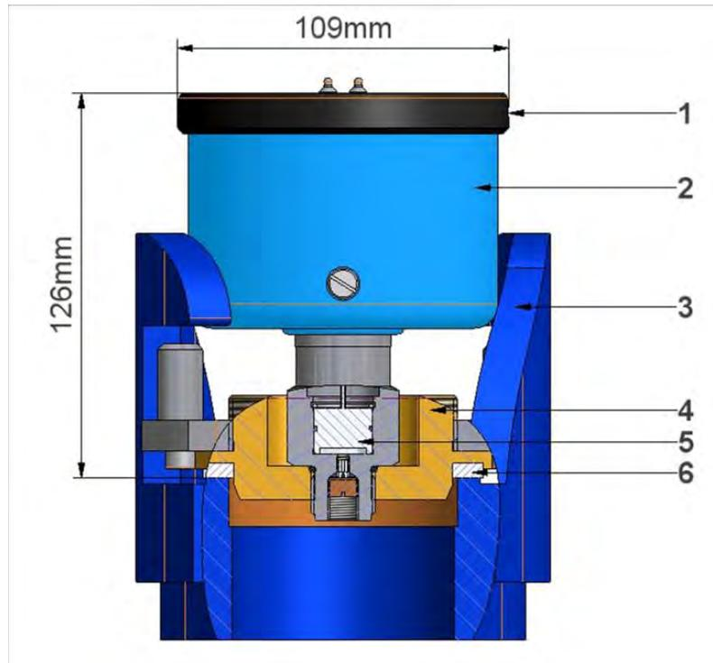
Figure 10: ESS3 water housing with bayonet adapter
