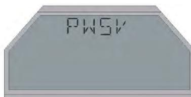
By pressing the button
