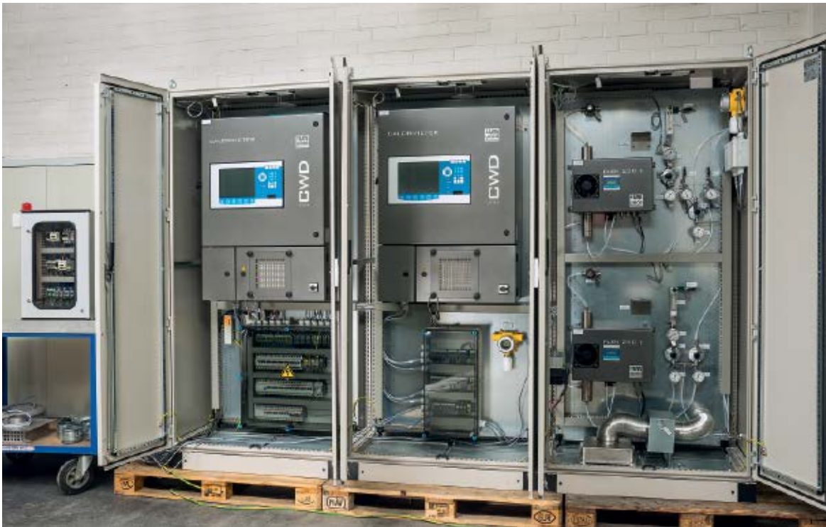
Calorimeters of the CWD series are used, for example, in glass production. There, they monitor the energy content of the combustion gas, thereby assuring the process control.
