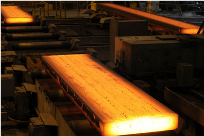
Fig. 1: Hot-rolling mill for steel production
